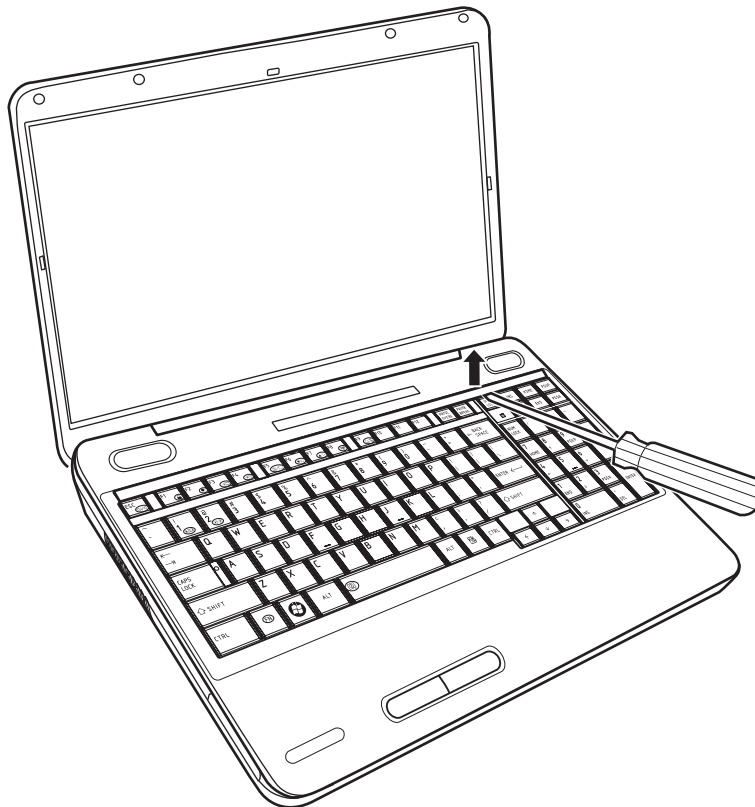
Figure 4.8 Removing the keyboard cover
